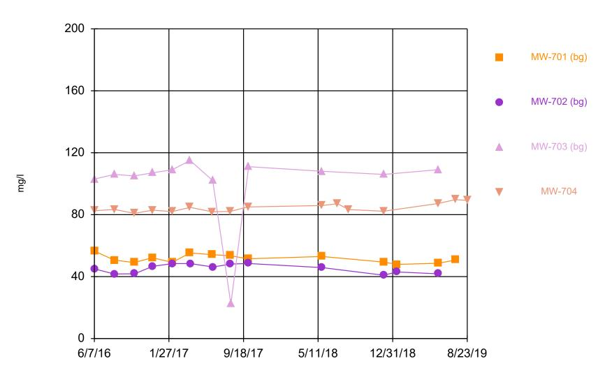
Constituent: CHLORIDE Analysis Run 10/30/2019 11:32 AM View: Bottom Ash III LaCygne Client: SCS Engineers Data: LaC GW Data
