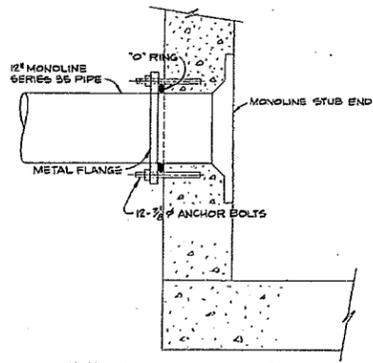
NOTE: COAT ALL EXPOSED STEEL WITH COAL-TAR PROTECTIVE COATING.
